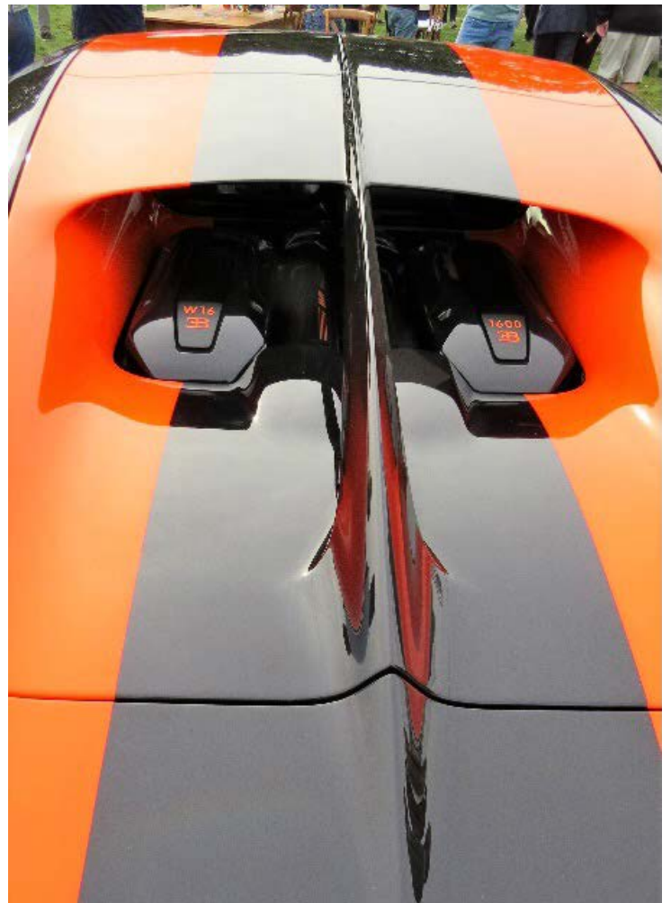
The Chiron is powered by an 8.0L W16 engine producing 1,500 hp.
